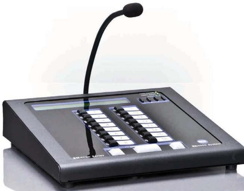
Digital paging console with 16/32/48/64 assignable keys, a general call 'A' key, a key to turn the chime on/off and the key 'Speech' to talk (after the chime).
