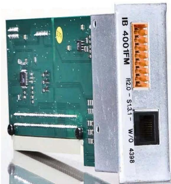
Emergency / fire microphone input for all calls and activation of 2 messages (or 3 zone paging). PTT, SW1, SW2 push-buttons can be monitored through 6.8k resistors between commands and the ground terminal.
