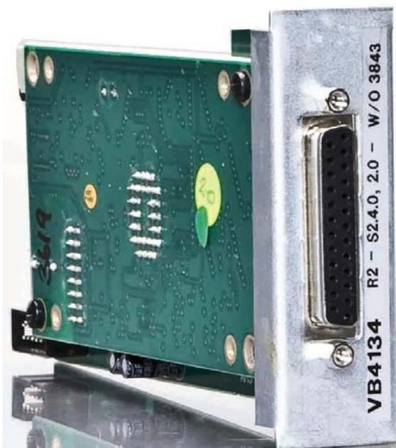
25 pin SUBD socket to be connected to a PC parallel port to upload the audio messages into the VB 4134 'flash' memory (by using the dedicated software)
