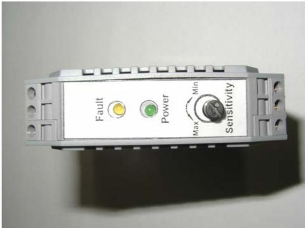
'END OF LINE' modules are always to be inserted when there are audio signal links from CP4100 to external devices (i.e. amplifiers).
