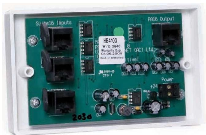
Expander board for 3 digital paging consoles (BM 4716, BM 4732, BM 4748, BM 4764).
