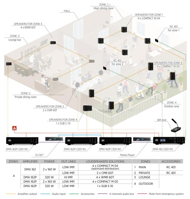
RCF provides examples of typical applications using various products as a general guideline, not intended as a reference for installers.
