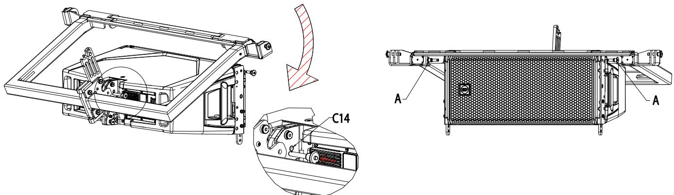
Fix the Link Bar HDL50-30 to the HDL30-A rear bracket using the inclination hole marked as C14 °.
