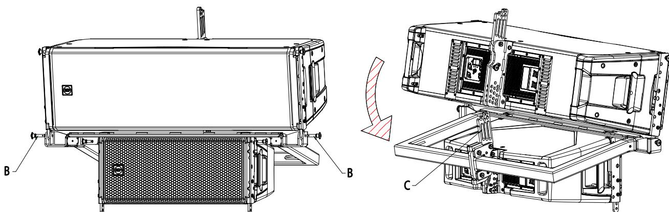
Fix HDL50-A in its front side using the quick lock pins "B".
