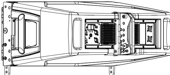
Max 8 HDL30-A modules hanged. Set the HDL30-A rear bracket as shown in the image (rest position).
