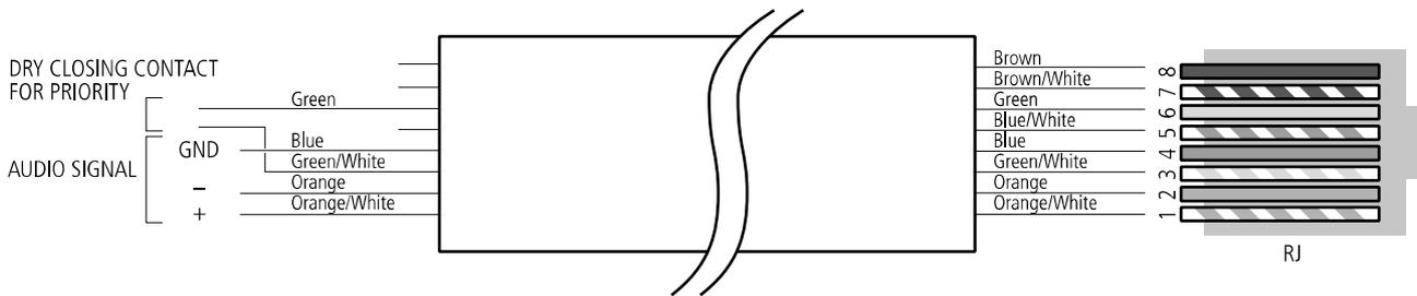
[3] **BGM IN** balanced audio input normally linked to the internal MP3 player, but also assignable to an external background music source (e.g. CD / MP3 player, tuner, etc.).
