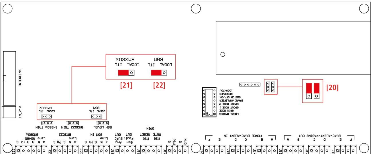
1. Check the jumpers [20] are corrected inserted in the position shown in the picture.
