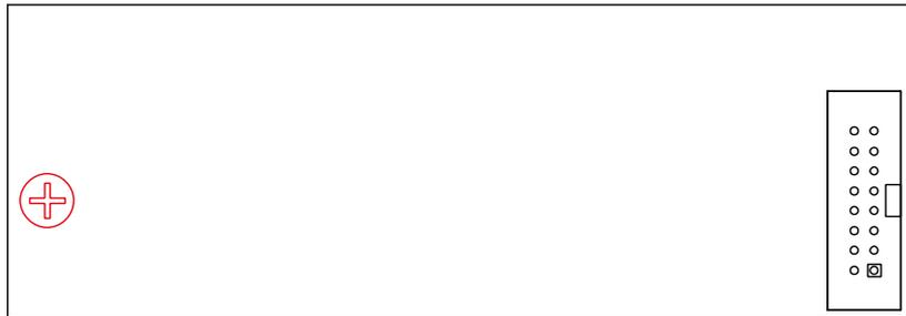
Remove the screw marked in RED to access the SD CARD and manage the messages.
