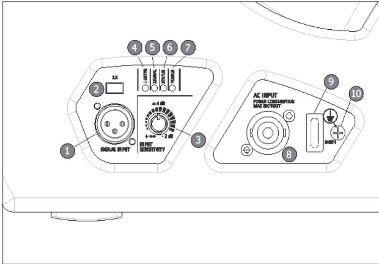
**TT45-SMA SIGNAL INPUT PANEL AND AC INPUT PANEL**
