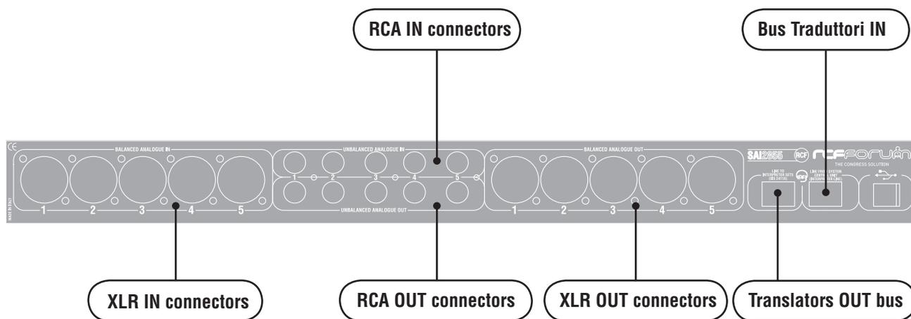
The codec unit must be connected to the interpreter consoles line in the same way as a console (there are thus no particular constraints).
