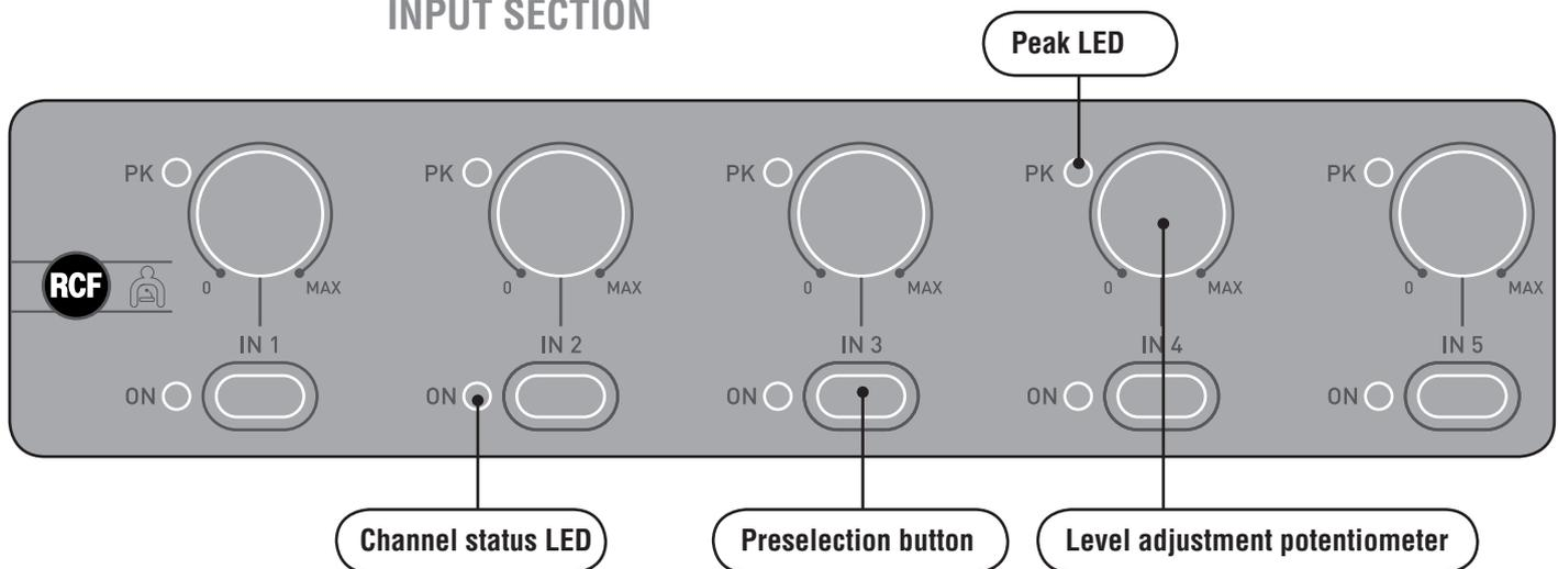
Each input channel has a dedicated set of controls. The channels are numbered from 1 to 5 starting from the left and refer respectively to the 5 languages assigned to the translator bus to which the codec unit is connected. If, for example, an audio track has to be inserted on channel 4, the fourth group of controls from the left must be used.
