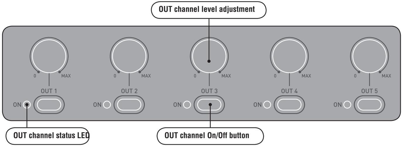
The output section is similar to the input section, apart from the absence of the level indicator LEDs.
