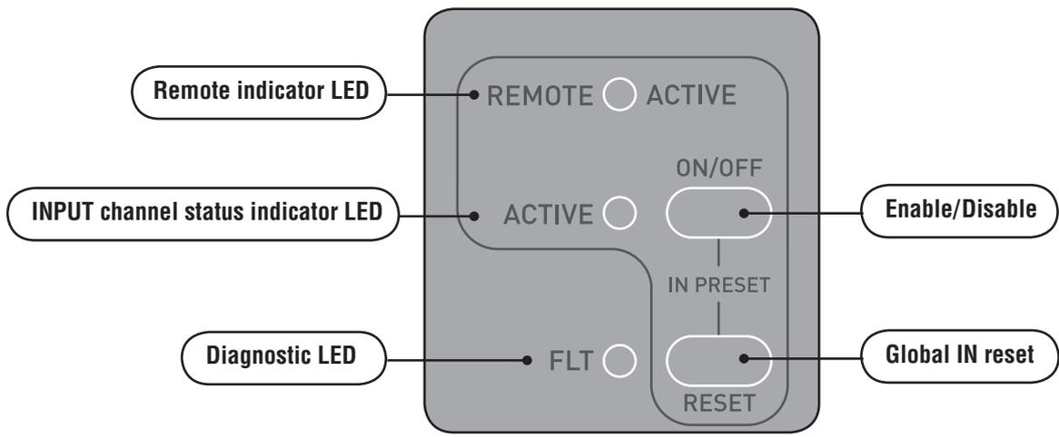
In the central zone the red LED at the top indicates, when on, that the device is operating in remote mode, which means that it is controlled remotely (a function currently not available). If the LED is off then the local controls are enabled.
