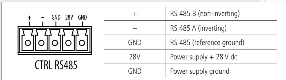
**33<sup>a</sup> FLEXCOM BUS IN:** data bus input (removable connector).
