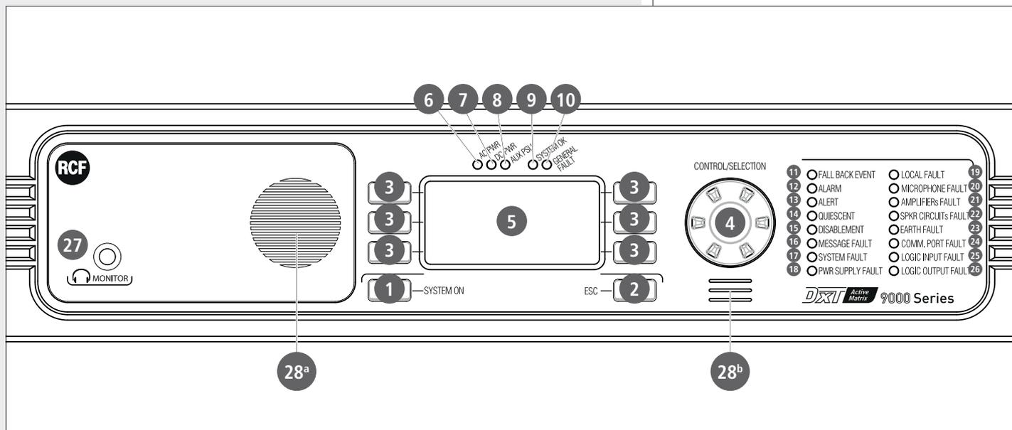
**1 SYSTEM ON** button: press and hold to turn amplifier on (when off). This button also works as fault acknowledge: press it to remove the displayed fault indication.
