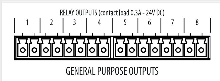
Each logic output has two resistors that can be inserted by setting the respective jumper (JP1 to JP8) to the **AB** position. These two resistors are necessary when the logic output (**GPO**) is linked to a logic input (**GPI**) of another device and the line monitoring is required.
